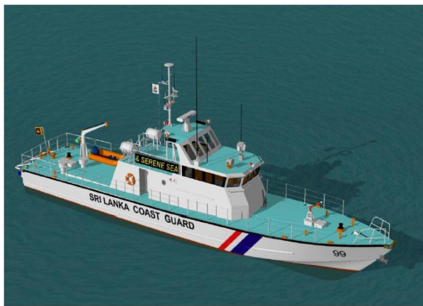
1,440 kW diesel powered patrol vessel
